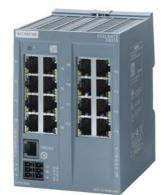
SCALANCE XB216 managed Layer 2 IE switch, 16X 10/100 Mbit/s RJ45 ports, 1x console port, diagnostics LED redundant power supply IEC 62443-4-2 certified; temperature range 0 °C to +60 °C; DIN-rail mounting, PROFINET IO device Ethernet/IP certificate, default PROFINET.
