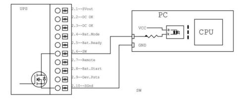
When the NP-6310 works in the load current monitoring mode, if the load current is lower than the set threshold (set by the rotary switch), the SW will output a pulse signal, whose pulse width time\_h can be set by Modbus register 40013.
