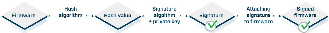
Before being installed on the device, the new firmware is verified. To ensure that the new firmware has not been tampered, the corresponding public key stored inside the Secure Element of the device is used to confirm that the hash value was indeed signed with the matching private key. By also computing the hash value of the firmware and comparing it to this validated hash value from the signature, the integrity of the firmware can be verified.
