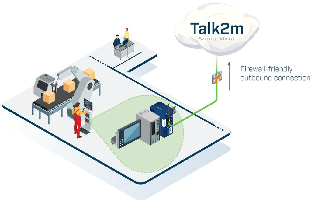
One effect of connecting to the Internet from inside a LAN is the possibility of having to pass through HTTP proxies. This will require proxy authentication settings to be provided in the Ewon gateway configuration or/and in the Ecatcher configuration. Proxies that are supported by both Ecatcher and Ewon gateways are:
