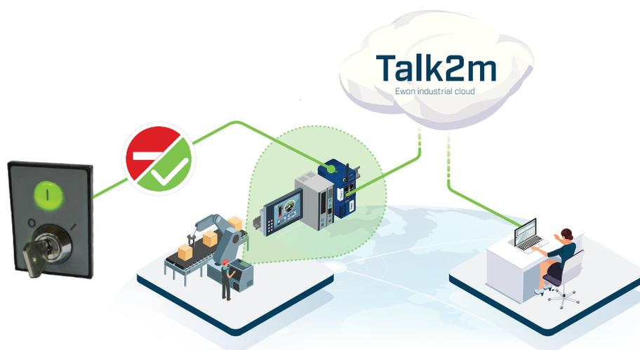
In some cases, it can also be preferable to keep offline Ewon gateways equipped with modem and connecting to the Internet through a cellular network, in particular to save on SIM card data traffic costs. For isolated equipment with nobody around to manipulate a key switch, this can be achieved by configuring the Ewon gateway to use a “triggered” connection.
