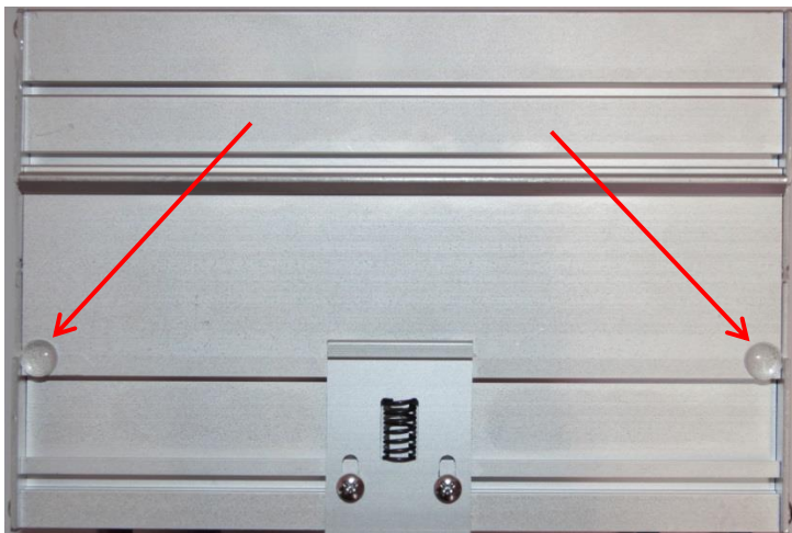
Fig. 9 – Rubber studs on backside of housing
