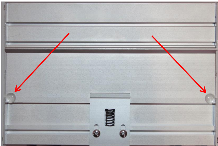
Fig. 9 - Rubber studs on backside of housing
