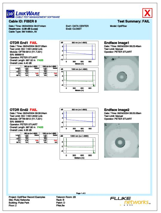
Figure 5. Fiber Cable Report from OptiFiber Tester, Page 1
