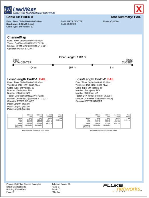
Figure 6. Fiber Cable Report from OptiFiber Tester, Page 2
