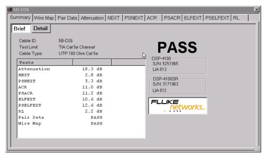
Figure 2. Results Pop-up Window (copper results shown)
