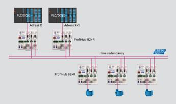
If bus redundancy is enabled, 2 segments will form a redundant pair. Short circuit protection on each spur line is automatically provided.
