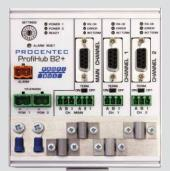
The ProfiHub B2+R is equipped with 2 galvanic isolated transparent repeaters (offering 3 segments). This allows network structures with extended spur lines that individually can handle up to 31 devices and a length equal to the main bus. To save costs on plugs
