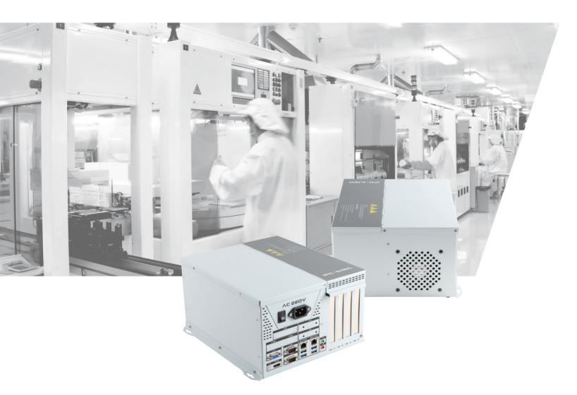
IPC615G based on Intel Core 6/7/8/9 generation i7/i5/i3,Pentium and Celeron LGA1151 desktop processors, 2 SODIMM slots support up to 32GB memory, with 1 Mini SATA interface and 1 2.5" HDD storage socket slot; VGA/HDMI supports synchronous or asynchronous dual display. equipped with rich I/O interfaces, 2 Gigabit Lan, 4 USB3.0/2.0/1.1, built-in 1 USB2.0, 2 RS232 or RS485 and also provides 2 PCI and 2 PCIe expansion slots which is convenient to expand a variety of function cards.
