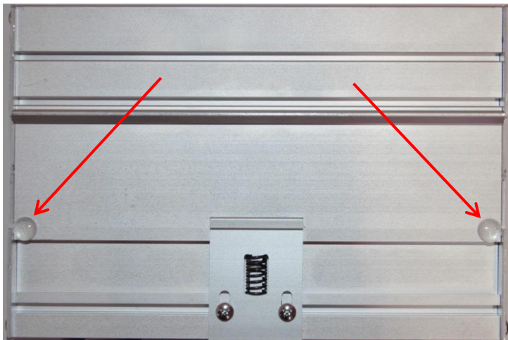
Fig. 9 – Rubber studs on backside of housing
