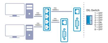
The HUB mode is determined via the DIL switch block on the back of the switch by setting switch five to ON.
