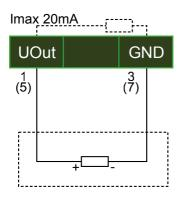
You may also connect this Sense line externally. This is recommended especially for longer cable routing.
