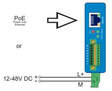
At a typical supply voltage of 24V the Web-IO draws approx. 100mA of current.
