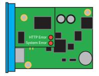
HTTP Error: Indicates internal errors in the configuration. For troubleshooting open the page http://xxx.xxx.xxx/diag in the device.
