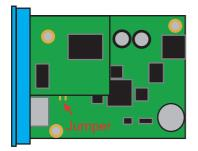
Close the jumper and power up the Web-IO for approx. 30 seconds. The Web-IO is now configured with its factory default settings.
