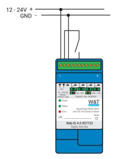
Alternatively, an external voltage of max.  $\pm 24V$  DC can be applied to the plus terminal, whereby voltages greater than 8V ( $\pm 10V$ ) are recognised as ON signal. In this case, the reference ground must be applied to the respective minus terminal.
