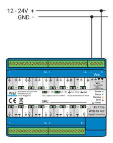
With a voltage supply of 24V, which is typical in industry, the Web IO draws approx. 100mA current.
