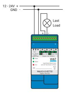
When connecting inductive loads such as relays, a free-wheeling diode is absolutely necessary to protect the internal circuitry of the Web IO from overvoltage.
