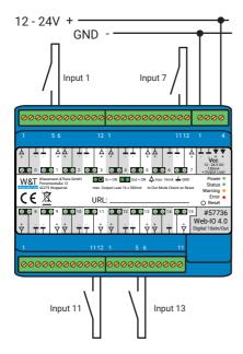
Alternatively, an external voltage of max. +24V DC can be applied to the plus terminal, whereby voltages greater than 8V (+/-1V) are recognised as ON signal. In this case, the reference ground must be applied to the respective minus terminal.
