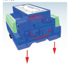
Use a pointed object to press on the latching hooks on the side of the housing and at the same time pull the bottom of the housing out of the top shell.
