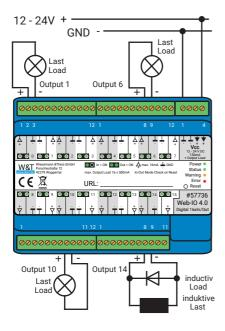
When connecting inductive loads such as relays, a free-wheeling diode is absolutely necessary to protect the internal circuitry of the Web IO from overvoltage.
