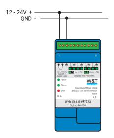
With a voltage supply of 24V, which is typical in industry, the Web IO draws approx. 100mA current.
