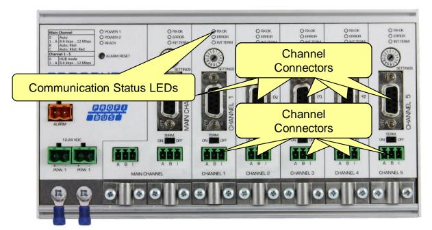
Figure 9 - PROFIBUS DP spur connectors
