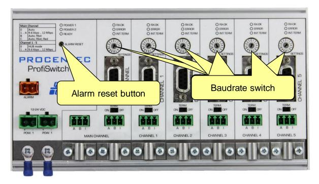
Fig. 16 – Baudrate speed switch
