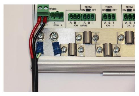
Fig. 12 – Connection to Ground Rail
