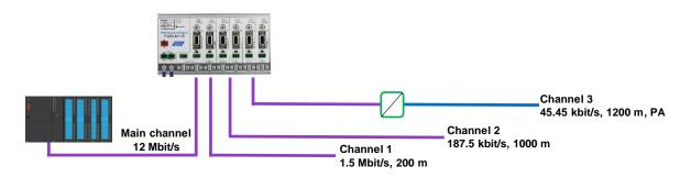
Figure 3 - Application example: One network, multiple baudrates, different cable lengths
