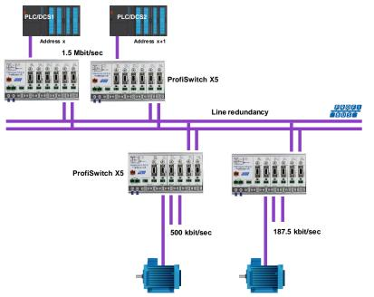
The telegrams are transferred onto both redundant channels. The logic inside the ProfiSwitch determines which telegram is used to be transferred onto the other channels. A message received by a redundant path is repeated on all other channels, except the other redundant channel. A message received by a normal channel is repeated on all other segments.
