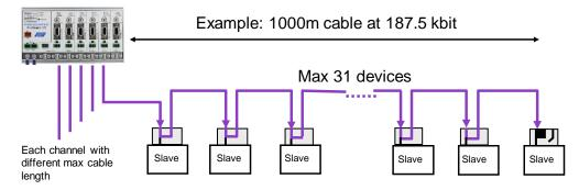
Figure 5 - PROFIBUS cable lengths and baudrates
