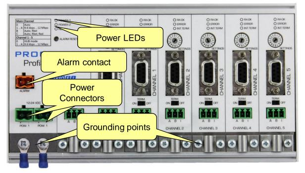
Figure 7 - Power connectors and LEDs
