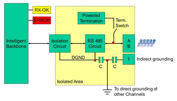
Figure 4 - Channel structure
