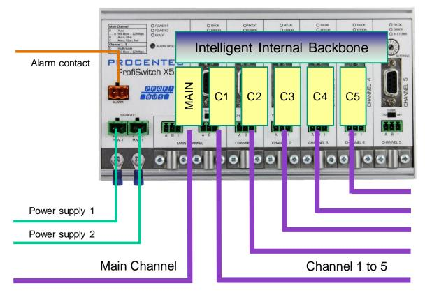
Figure 2 - Connections of the ProfiSwitch X5
