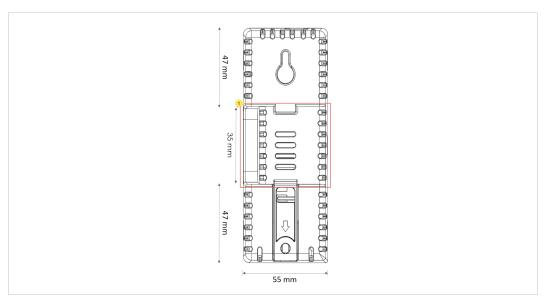
Fig. 3 DIN rail mounting position
