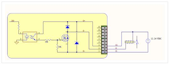
Fig. 17 External wiring for the Digital Output
