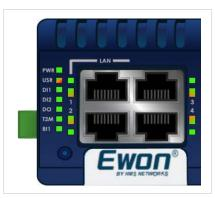
Fig. 9 LED Panel Example of a Flexy 205
