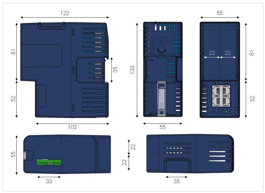
Fig. 7 Mechanical Dimensions
