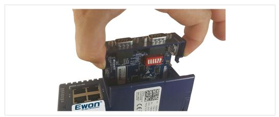
Fig. 13 Slot Removal
