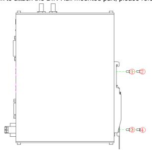
Figure 9 Attach DIN-Rail mounted part
