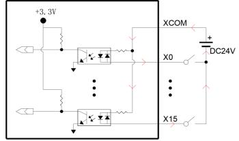
Figure 6 DI NPN wiring solution
