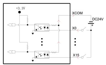
Figure 7 DI PNP wiring solution
