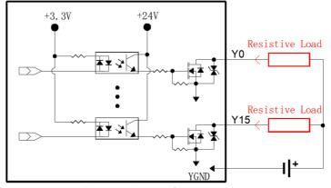
Figure 4 Wiring of resistive load
