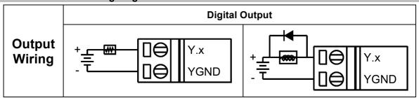
Figure 13 DO electrical wiring diagram
