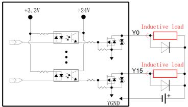
Figure 5 Wiring of inductive load
