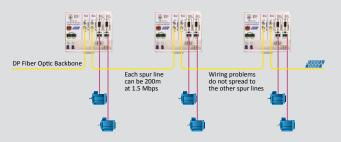
Long spur lines to instruments and the possibility to remove/insert them during operation. Short circuit protection on each spur line is automatically provided.
