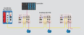
Creating a fiber optic backbone increases network reliability and network overview. It is also possible to mix ProfiHubs with ComBricks.
